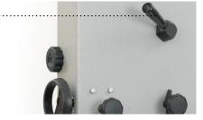
Cam Action Tensioner With the flick of a handle the tension is released on the blade enabling quick easy changing, but more importantly, when reset, the previous tension is automatically applied to the new blade. This makes blade changing a much simpler task and allowing tension to be taken off the blade when not in use.
