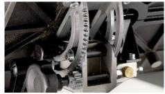
**Trunnion** Solid double trunnion table mount for rigid table support featuring one handed rack and pinion table tilt for ease of use and accuracy. Mounted on top of bandwheel box with jacking screws for easy adjustment.
