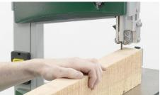
Capacity Large 120 mm depth of cut and 240 mm
