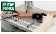
Table A solid, finely ground cast iron table provides an ideal and low friction work support.
