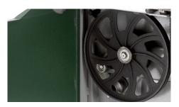
Cast Iron Band Wheels Are dynamically balanced and provide a flywheel effect for improved cutting performance. Rubber tyres are precision ground for easy blade fitting and smooth drive. · · · · · · · ·
