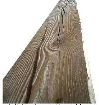
A valid system for personalizing wood products is **brushing.** This operation consists in modifying surfaces, highlighting the grains of the wood. In point of fact, it is simply a matter of "bringing out" what is already there in the wood, i.e., the natural wood-grain pattern which gives a very beautiful natural appearance.
