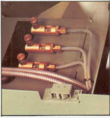
Cleaning fluid accurately controlled by drip feed valves with automatic cut-off device.
