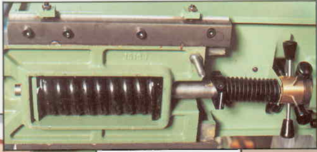
Heavy duty support column for top saw wheel with sensitive tensioning system. Substantial steel fabrications throughout.
