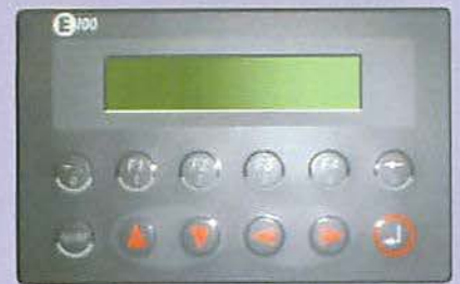
HMI Control Unit
