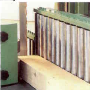
True radial arm feed gear and multi-roller fence for accuracy.
